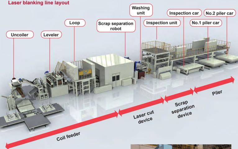
Laser blanking line is a line that press machine is replaced with laser cut device in traditional blanking press line consisting of coil feeder, press and piler.
